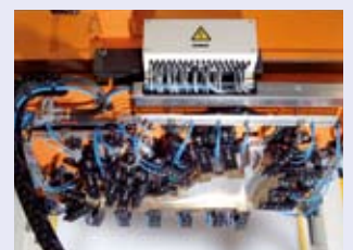
Press laminating with edgelifting, combi tool
