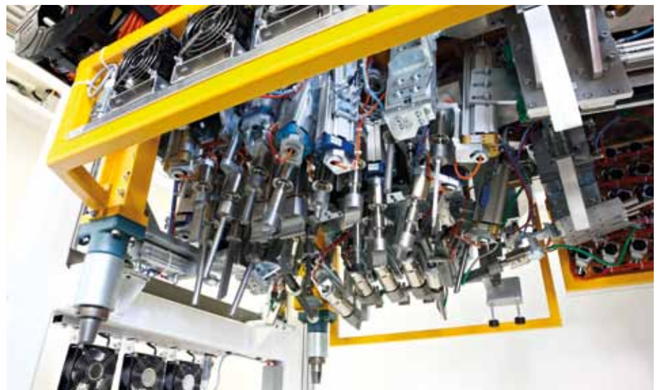
Complex ultrasonic joining tool with ultrasonic standard components
