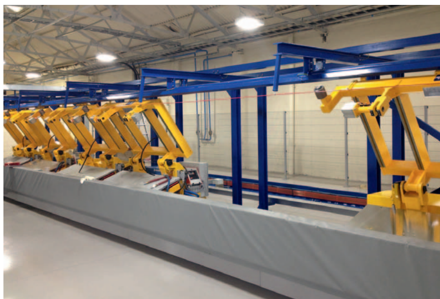
Fig. 2. Combination of four mold carriers with a single drive in the operating area
