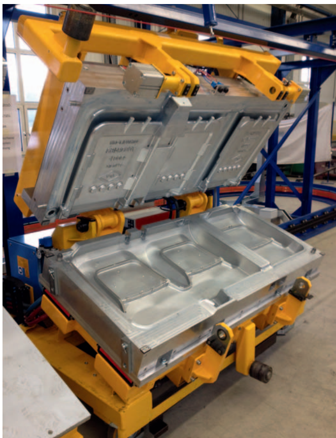
Fig. 1. Mold carriers guided by the low monorail traversing the shop floor
