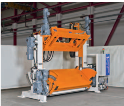
Fig. 3. Mold carrier for evaluating RTM components with Vitrox in the pilot plant. The picture sequence shows important swiveling functions (figure: Frimo)
