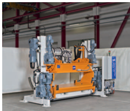
Fig. 3. Mold carrier for evaluating RTM components with Vitrox in the pilot plant. The picture sequence shows important swiveling functions (figure: Frimo)
