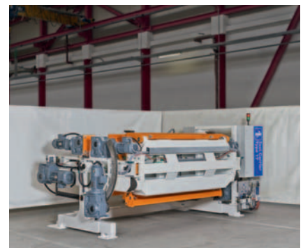
Fig. 3. Mold carrier for evaluating RTM components with Vitrox in the pilot plant. The picture sequence shows important swiveling functions (figure: Frimo)
