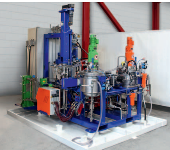
Fig. 5. Ultra precise, high-pressure two-component dosing machine as required for the pilot plant, and adapted to the processing of Vitrox (figure: Frimo)
